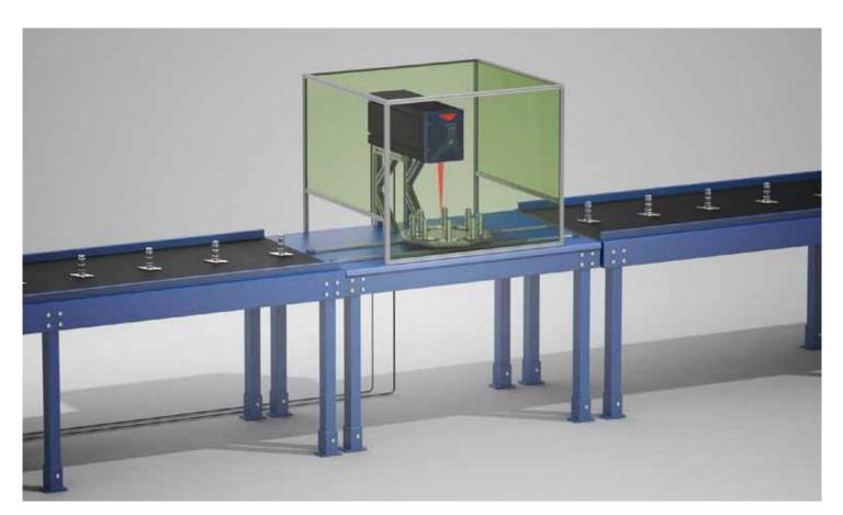
UniQ<sup>™</sup> do not requires any additional external unit. Integration in production lines is simple and quick and involves only power supply, Ethernet and I/O signals.
